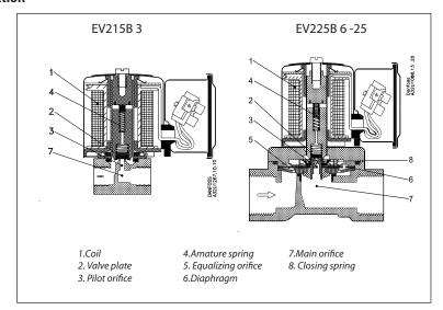
Coil voltage disconnected (closed):
